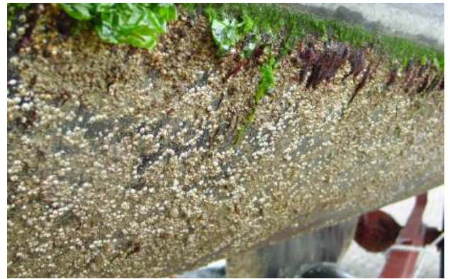
Macrofouling on a motor vessel
