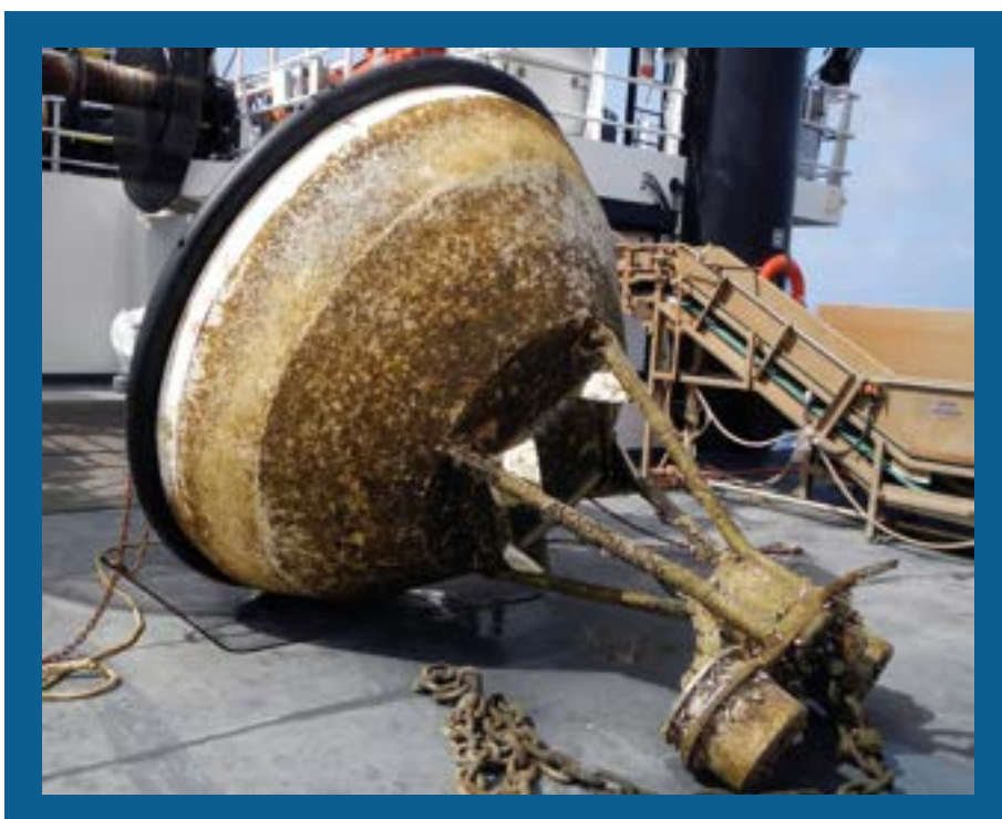
Figure 2-10: NOAA dart tsunami warning buoy recovered for cleaning and maintenance
