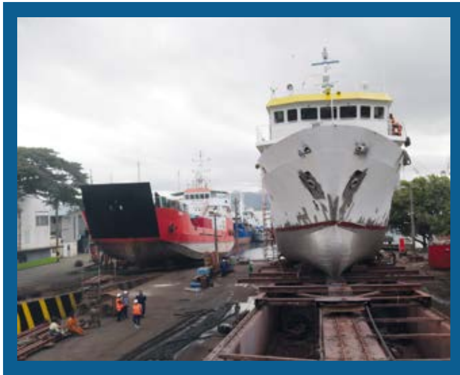
Figure B-2: Example of a slipway and haul out facility
