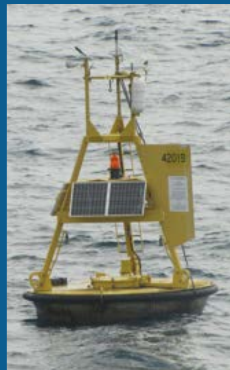
Figure 2-9: Floating meteorological monitoring buoy
