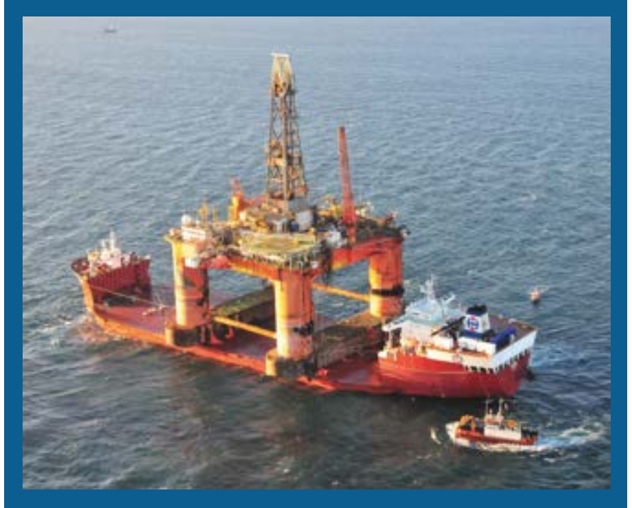
Figure 2-7: Semi-submersible drilling rig being transported
