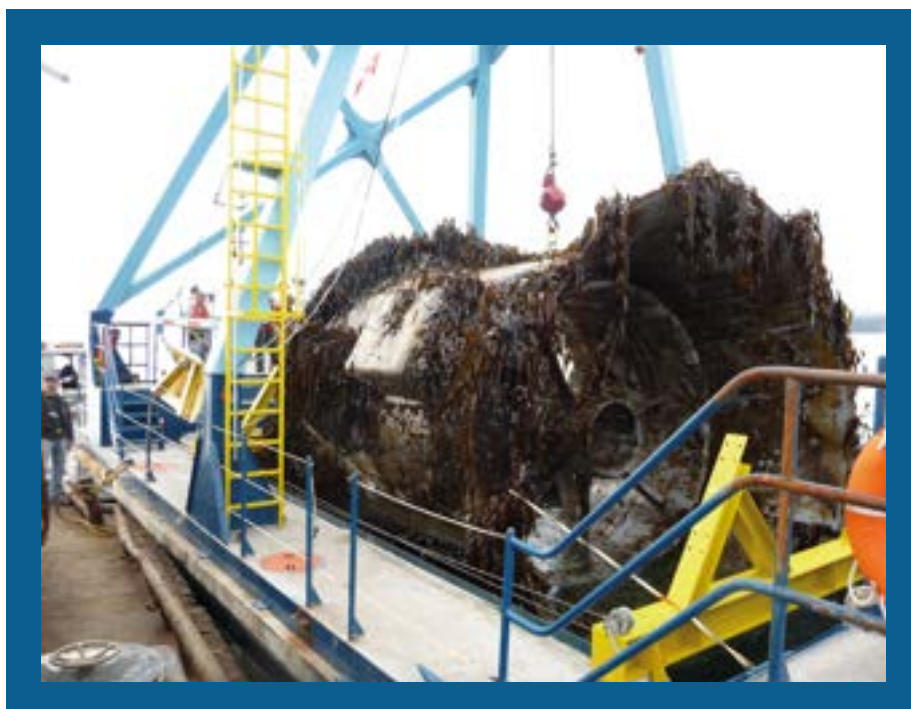
Figure 2-16: Macro-algae fouling on a tidal turbine
