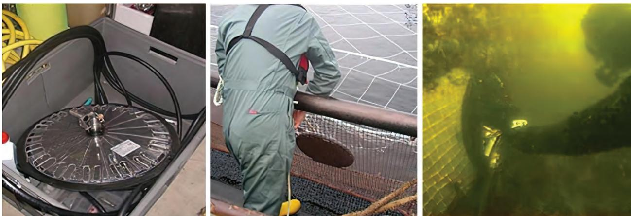
**Figure 8.** From left to right: a basic disk washer, a disk washer used from a supporting vessel, a disk washer used by a diver. (photos: Left Simone Durr, middle and right Collective Research on Aquaculture Biofouling (CRAB), 2006)
